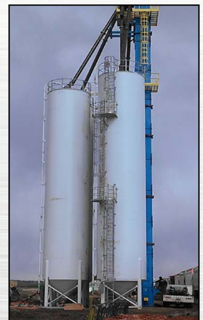
(3) 12' x 48' Factory-welded and epoxy coated tanks for portable Frac Sand storage.
