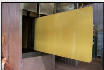
Tank panel being conveyed through 400 degree curing oven.
